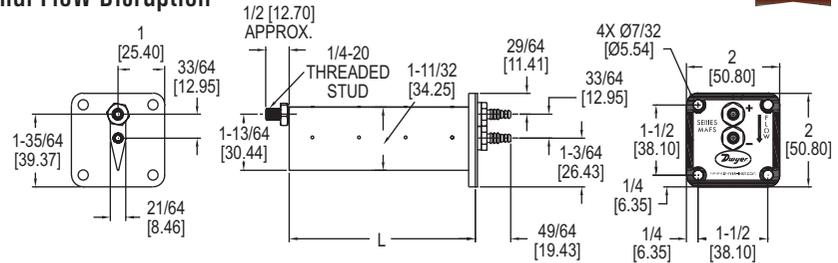
The **Series MAFS Metal Averaging Flow Sensor** is ideal for use with Dwyer Instruments, Inc. precision air velocity gages, transmitters and switches. The Series MAFS uses evenly distributed total and static pressure measuring points to deliver an accurate measurement of velocity pressure in a duct.
