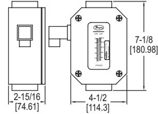
The **SERIES HFT** In-Line Transmitters provide continuous monitoring of flow rate levels via a direct reading in-line flowmeter with electronics to provide proportional 4-20 mA, 0-5 and 1-5 VDC analog outputs.
