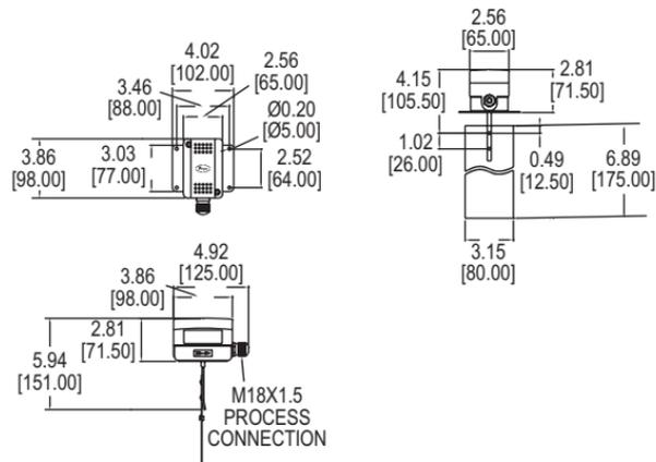
The **MODEL AAFS** Adjustable Air Flow Switch is capable of detecting a wide range of air velocities with minimal user calibration. Quality features include a stainless steel vane, galvanized steel base, and ABS enclosure.
