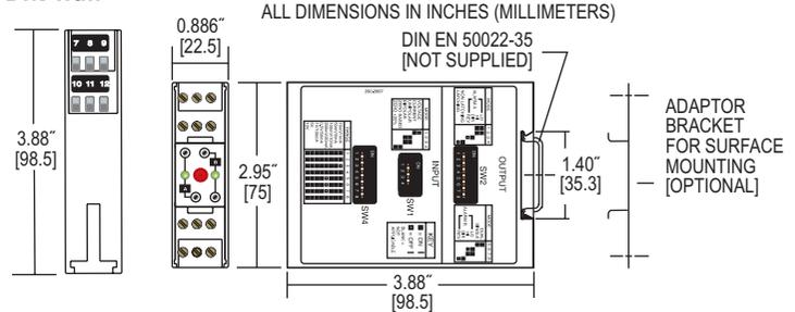
The **SERIES SC1** Limit/Alarm Switch Modules are on-off or limit switches with selectable process signal. Each unit has two form C (SPDT) relays which can operate independently, or be logically connected to operate as a DPDT output.
