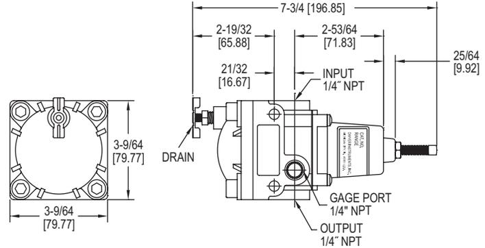
**SERIES AFR** Air Filter Regulator provides clean air pressure to pneumatic controllers, valve positioners, air cylinders and other equipment. Self-relieving regulator is equipped with a 40 micron filter housed in a dripwell with gage port.
